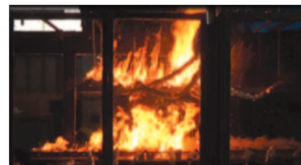
Figure 9: Class E Experiment. Flame velocity and overall intensity is substantially higher due to addition of surface fuel and wind parameters.
