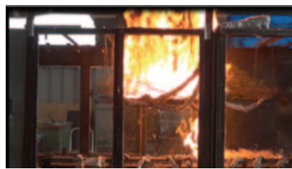
Figure 8: Class C Experiment. The propagation of crown flame is furthered by addition of surface fuel.
