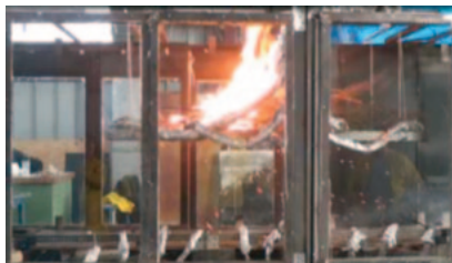
Figure 7: Class B Experiment. Flame velocity and fuel consumption rate rise significantly due to added wind.
