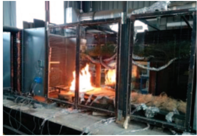
Figure 1: Live burn being conducted on chamise (Upper platform) by ignition of excelsior (lower platform) inside of the wind tunnel.
